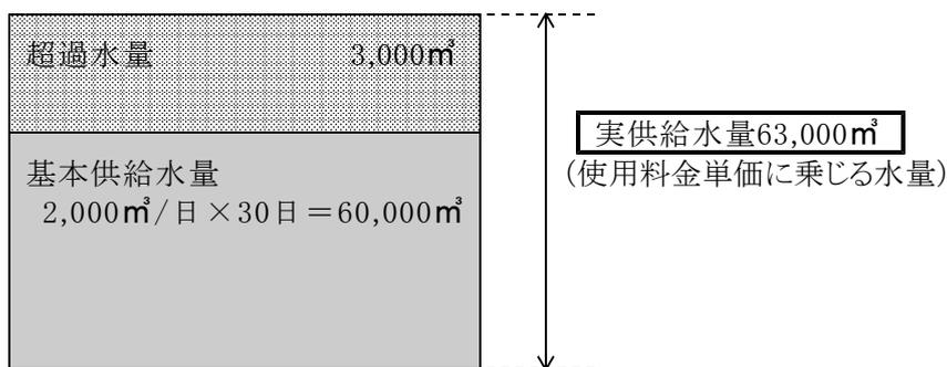
$$\begin{aligned} \text{1ヶ月の料金} &= \text{基本料金} + \text{使用料金} + \text{超過料金} + \text{消費税及び地方消費税相当額} \\ &= (2,963,400 + 564,480 + 304,020) \times (1.10) = 4,215,090 \text{円} \\ \text{基本料金} &= 49.39 \text{円/m}^3 \times 60,000 \text{m}^3 = 2,963,400 \text{円} \\ \text{使用料金} &= 8.96 \text{円/m}^3 \times 63,000 \text{m}^3 = 564,480 \text{円} \\ \text{超過料金} &= 101.34 \text{円/m}^3 \times 3,000 \text{m}^3 = 304,020 \text{円} \end{aligned}$$
